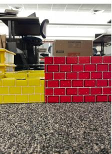
The yellow bricks are half the height of the red bricks, so position the ultrasonic sensor on the base such that it can see the red, but not the yellow when it drives close. This way, yellow can indicate one direction to turn and red can indicate the other direction to turn.
